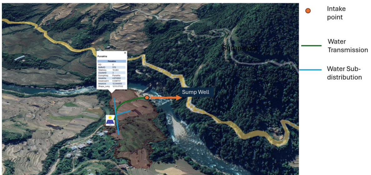
Figure 1. An example of an individually owned solar PV pumping system designed to efficiently extract water and distribute it to nearby clusters, thus enabling sustainable water access and income generation through local water sales.
